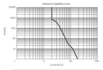
Note: The above data is tested at 85 °C ambient temperature, connecting wire cross section area≥4mm². The data is for reference only; please do not use to select the fuse directly.
