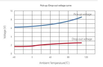
Note: The above data are tested by random sampling of coil volt. 12V DC product. The data is for reference only, (test qty: n=3)
